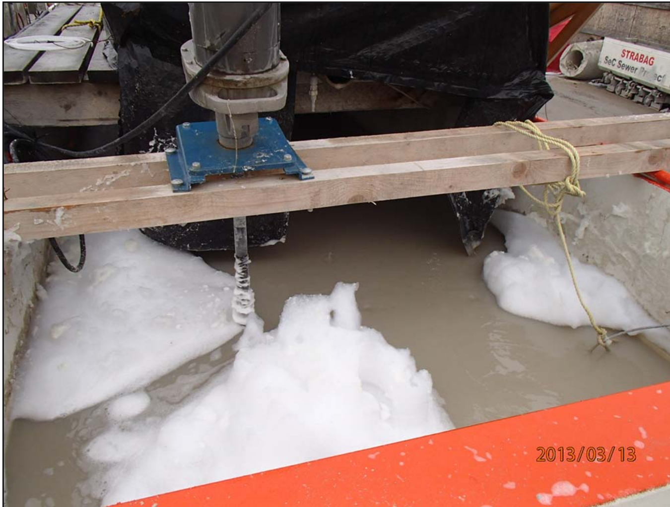
Acid dosing drip tube and nipple (right) and mixer (left)
