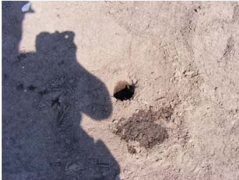
Infiltration Testing During Construction: 50–75mm/hr
