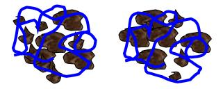
Flocculation is the process where a chemical agent (flocculant) is used to reduce the turbidity of a liquid by binding suspended particles in the liquid together to form larger particles (flocs) that are heavy enough to settle to the bottom of the liquid.....Polymer flocculation provides the basis for a number of best management practices (BMPs) for reducing turbidity and its toxicity.
