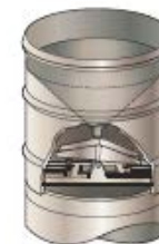
MSC Tipping bucket rain gauge — recording (TM 04-01-03, Environment Canada, 1981)
