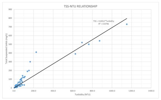
Figure 1. Relationship between Total Suspended Solid (mg/L) and Turbidity (NTU). The line represents the linear regression
