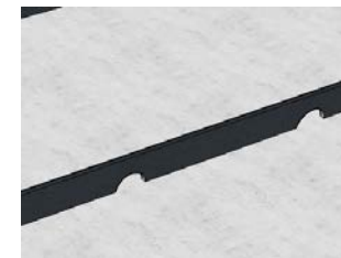
Blue Roof Check Dams Orifices
