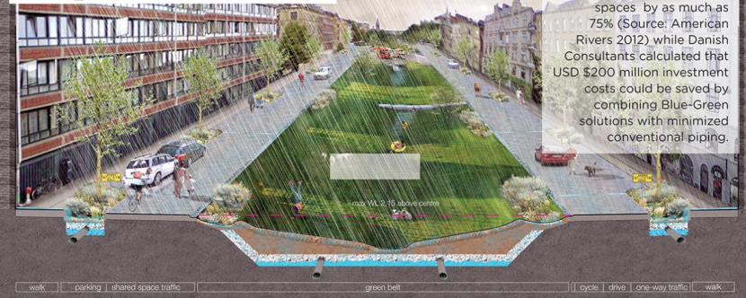
Rain Event Handled within Multi-Functional Tools including Urban Creek, Retention Boulevard, and Boulevard
